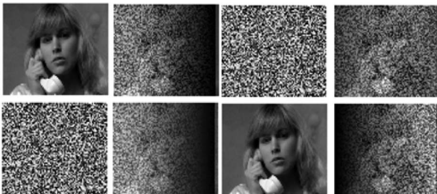
Fig. 10. Results of blind de-mixing for linear space-variant imaging problem. From left to right are: (a) source images; (b) space-variant noise free linear mixture; (c) recovery of the source images using Cauchy annealing based linear blind inversion algorithm described in Section 3; (d) recovery of the source images using Infomax ICA algorithm [6]. Due to the space-variant nature of the mixture that changes from pixel to pixel, stochastic ICA algorithm gave poor result.
